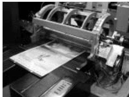
A.B. Dick's chemical free Vector CTP system with the "thin drum."
