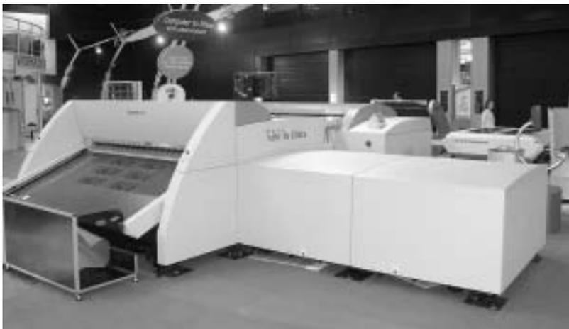
The Screen PlateRite Ultima 32000 images plates from 4-up to 32-up, with one GLV exposure head up to 30 8-up plates per hour. With two GLV heads, it is named Ultima 32000Z and images simultaneously up to 46 plates 8-up plates per hour or 22 212.4-by-127.6-cm plates per hour.
