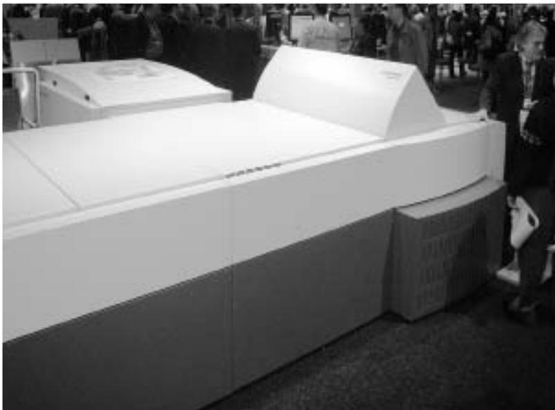
Heidelberg showed the new platesetter family SupraSetter, a completely new design with a new imaging head. The laser technology was developed by Heidelberg and the exposure module is a small box that easily will fit into platesetters or printing presses.
